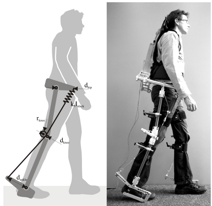
Figure 1. Left: Schematic drawing of the exoskeleton concept with artificial tendons (black). Right: A photo of the exoskeleton
